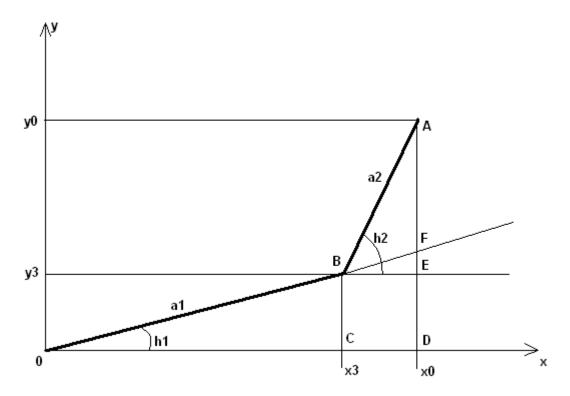
A scheme of simple manipulator is shown in Fig.1. It is required to determine the size h1 of BOC angle and size h2 of ABE angle. They will be calculated by using the expression (1).
